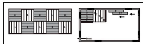
**IMPORTANT:** We recommend to apply a high-grab high-shear hard-setting adhesive inside the locking system at the short side of the planks for additional engagement, avoid using adhesive excessively and be sure to immediately wipe away any excess that comes out to the floor's surface.
